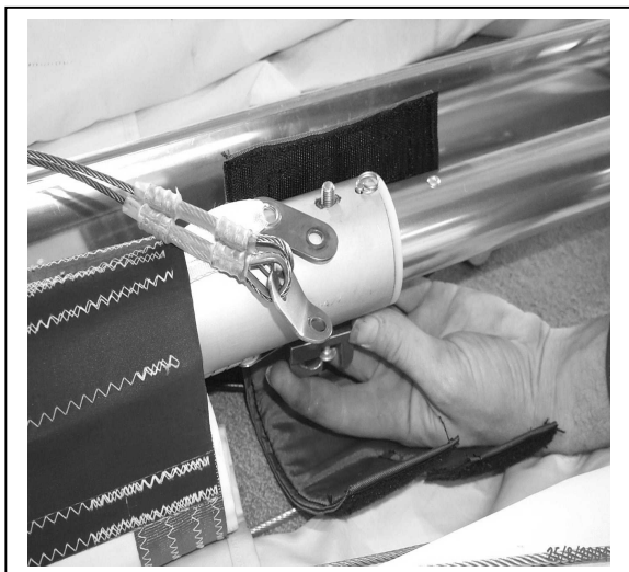
Figure 8 Removing Quick Clip Nut
