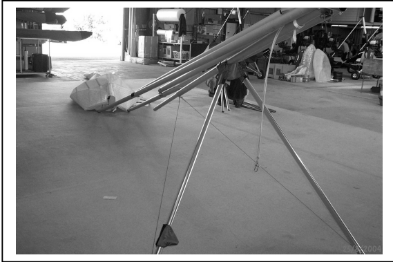
Figure 14 Frame Preparation For Sail Reinstallation
