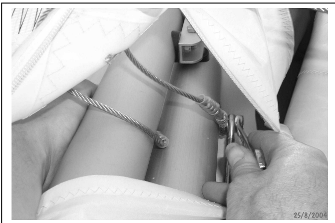
Figure 6 Unbolting Side Wires
