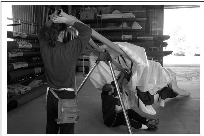
Figure 18 Position Keel Pocket Forward Of Rear Wires
