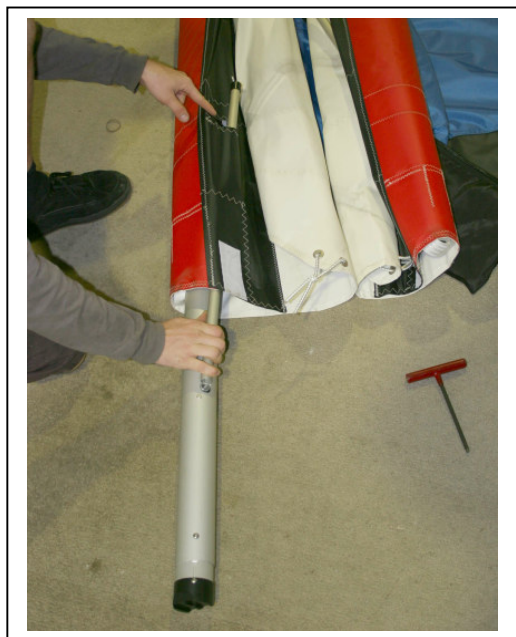
Figure 1 Insertion Of Rear Leading Edges
