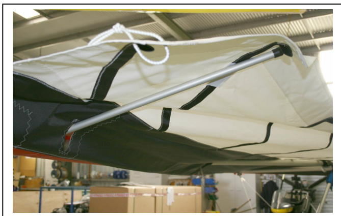
Figure 29 Insert Dive Stick Into Leading Edge
